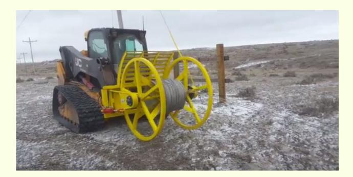
Abandoned high voltage power line has built up over years on NEA's system, as new lines have been built, becoming a hazard and an unfunded maintenance/tax issue. Removing such line has moved up on the list of priorities line crews are addressing this year, making the new wire winder a welcome piece of equipment.
